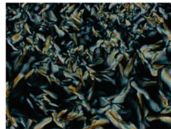
Figure 2. Polarizing optical micrograph of poly( I-4 ) (run 4 in Table 1).
